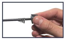
2. Remove the cap and one of the two springs from the quick release skewer.
