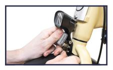
4. Connect the light cable. When mounting to the handlebars, attach with the included cable extender.
