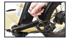
Start by handthreading each pedal onto the bike. Then, tighten the pedals securely using the 15mm crescent wrench.
