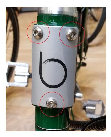
2. Attach The Front Basket: Line up the three holes on the Front Basket with the three holes on the head tube mounting point, and insert the three M8 20mm Screws (A), using one washer (B) each. Screw these in evenly using the 6mm Allen Key (D)
