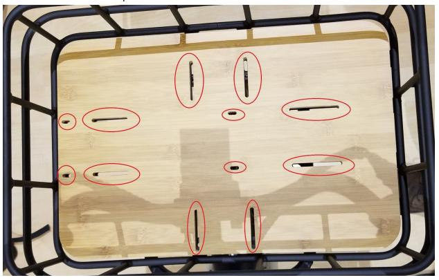
2. **Using the Large Basket on a Front Rack:** If you are installing the Large Basket on a front rack, line up 4 slots on the Basket to the holes on the front rack as shown in either of the two configurations shown below, and use the hardware included with the Front Rack.
