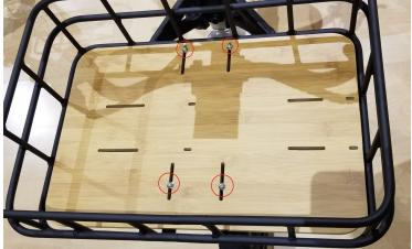
3. **Using the Large Basket on a Rear Rack:** If you are installing the Basket on a rear rack, line up the slots on the basket to 4 holes on the rear rack. Place the four 25mm M5 screws (A) in each hole using one washer (B) for each bolt. Screw these in evenly using the 3mm Allen Key (C). There are multiple configurations possible.
