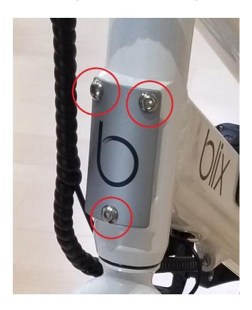
2. **Attach The Front Rack:** Line up the three holes on the Front Rack with the three holes on the head tube mounting point, and insert the three M8 20mm Screws (A), using one washer (B) each. Screw these in evenly using the 6mm Allen Key (I)
