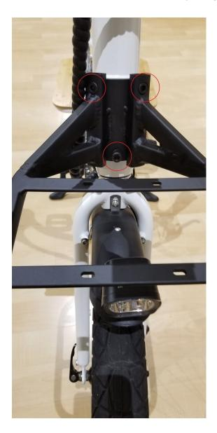
3. Additional Hardware: Use the additional hardware to install other accessories on the Front Rack. The M5 50mm Screws (C) can be installed on the front two holes, and the M5 30mm Screws (D) can be used on the four rear holes. To install these screws, use one washer (E) each, and one nut (F) each underneath the rack using the 3mm Allen Key (G) on the screw and the 8mm side of the Combination Wrench (J) on the nut.
