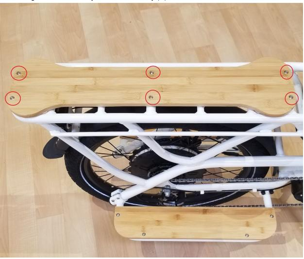
2. Connect the VIP Section to the Rack: Place the VIP section on the rear rack, lining up the four holes of the VIP Section with those on the rack rack. Insert the four 30mm M5 bolts (A) in the four holes, using one washer (C) on each bolt, and screw in each bolt evenly, using the 4mm Allen Key (E).
