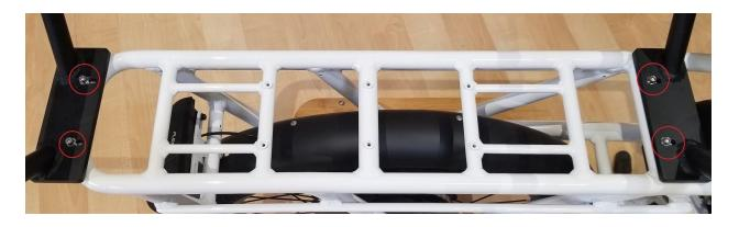
3. **Screw In the Water Bottle Bolts:** Insert the eight 12mm M5 bolts (B) in each of the eight water bottle bosses, using one washer (C) each, and screw in each bolt using the 4mm Allen Key (E). These bolts can be used to attach water bottle cages or other accessories to the sides of the VIP Sections!
