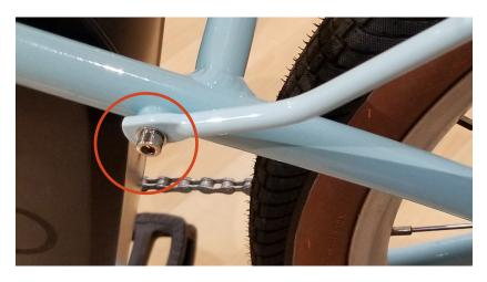
4. Attach the Strut to the Frame: Attach the strut to the mounting points on the frame using an M5 10mm bolt (D) and an M5 washer (F) on each side, and screw the bolts in using the 4mm Allen Key (M).
