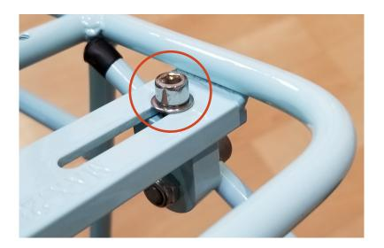
2. Attach the Strut Clamp to the Rack: Insert the M6 15mm Socket Bolt (B) through the top of the Rack using one M6 Washer (E), and screw the bolt into the top of the Strut Clamp Mount (A) using the 5mm Allen Key (L), ensuring the strut is on the outside of he rack. Repeat this for the other strut on the other side of the rack.
