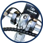
To adjust the **angle of the handlebar**, loosen the handlebar clamp. Ensure both bolts are tight once you have reached your desired wrist angle.
