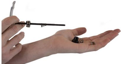
3. Push the quick release skewer through the axle of the front wheel from the side opposite the brake rotor disc.
