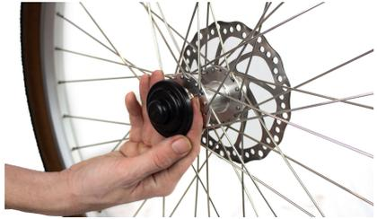
2. Remove the cap and one of the two springs from the quick release skewer.
