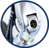
To adjust the **height of the stem**, loosen the stem bolt. Ensure the stem is fully aligned to the front wheel before tightening the bolt back down.
