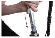
3. When the stem and fork are pointing forward in alignment, tighten down the stem bolt.
