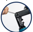
The stem angle can be adjusted by loosening the bolt on the side of the stem using the 5mm allen wrench. Adjust the stem to the desired angle, and secure tightly to ensure the position doesn't change or slip during use. This is the only bolt that should be loosened during adjustment.
