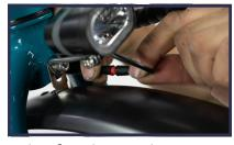
4. Attach the fender struts to the fender eyelets using the bolts removed in a prior step.
