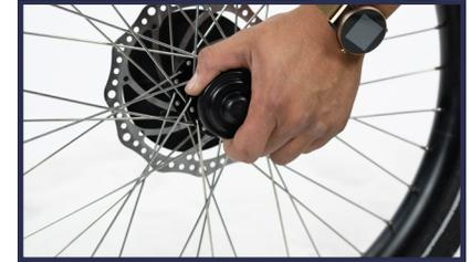
2. Remove the cap and one of the two springs from the quick release skewer.
