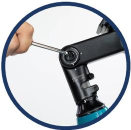
The stem angle can be adjusted by loosening the bolt on the side of the stem using the 5mm allen wrench. Adjust the stem to the desired angle, and secure tightly to ensure the position doesn't change or slip during use. This is the only bolt that should be loosened during adjustment.
