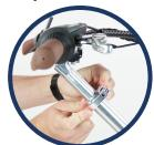
The handlebar height can be adjusted using the quick release on the stem. Adjust the stem to the desired angle, and secure tightly to ensure the position doesn't change or slip during use. This is the only adjustment that should be made to the handlebars when fitting your bike.
