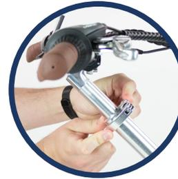
The handlebar height can be adjusted using the quick release on the stem. Adjust the stem to the desired angle, and secure tightly to ensure the position doesn't change or slip during use. This is the only adjustment that should be made to the handlebars when fitting your bike.
