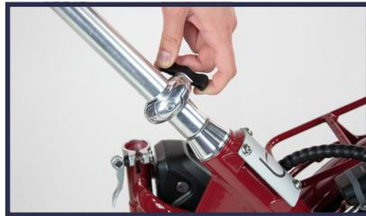
2. Insert the upper part of the handlebar stem into the lower handlebar stem of the bike.
