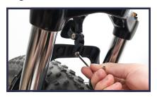
4. Connect the light cable. When mounting to the handlebars, attach with the included cable extender
